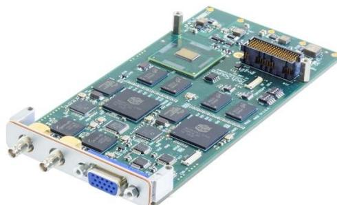
▲ Figure 4 The VC100x XMC H.264 encoder allows video to be sent remotely and in a timely fashion
